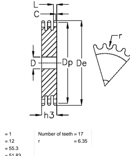
C = 1 D = 12 De = 55.3 Dp = 51.83 For chain size =  $3/8 \times 7/32$ For chain type = 06 B-3 h3 = 25.6 L = 5.2
